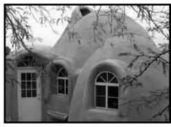
A finished superadobe home. An insulation of straw and then plaster are applied to the dome.
