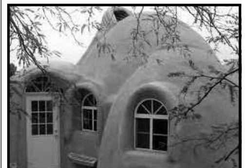
A finished superadobe home. An insulation of straw and then plaster are applied to the dome.
